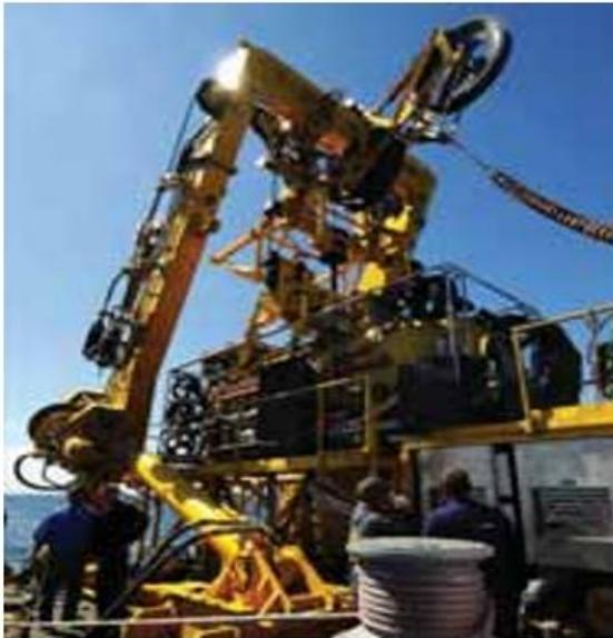
Gambar 10 *SRDRS launched using it's A-Frame*
